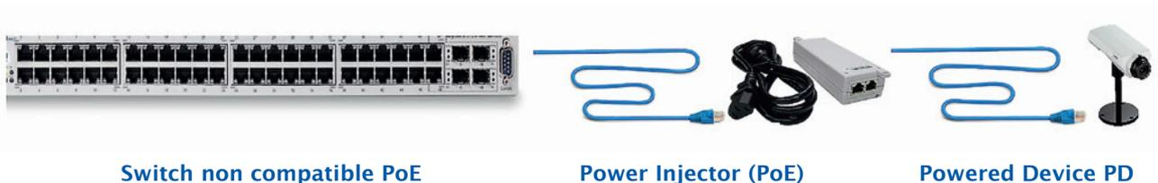
Figure 5 : Configuration PSE Mid-span
